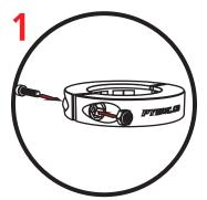
Pre-install the nuts on both collars by using the bolt to pull the nut into place.
