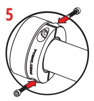
Tighten the assembly (alternating sides, back and forth) with the provided two bolts. *Snug, do not over tighten.*
