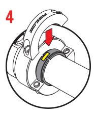
Apply tape to the ends of the rubber strip to hold it in place. Install the other half of the collar.
