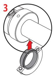
Install the rubber strip and collar assembly around the propeller shaft.
